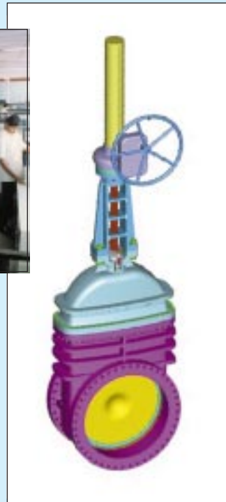
48" Class 150 Gate Valve - Pro/E Model & Actual Valve
