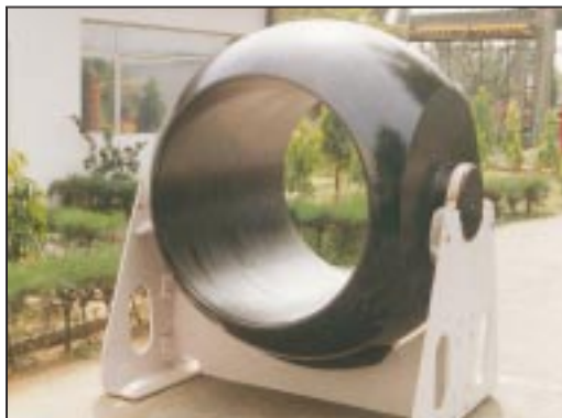
Precision machined 48" TMBV Ball
